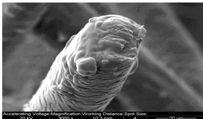
Figure 2 An SEM Image Of One End Of An Alpaca Fibre Strand (Magnification: 3000x, Working Distance: 10.3mm)
